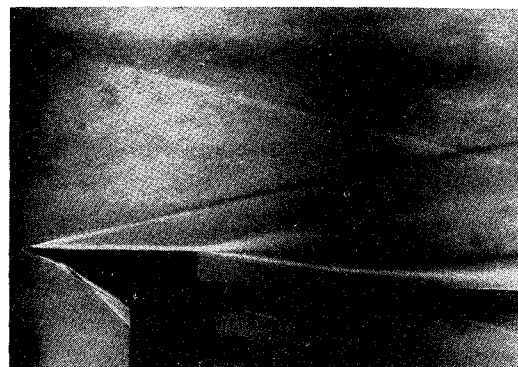
Fig. 2 Schlieren photograph of the flowfield.
